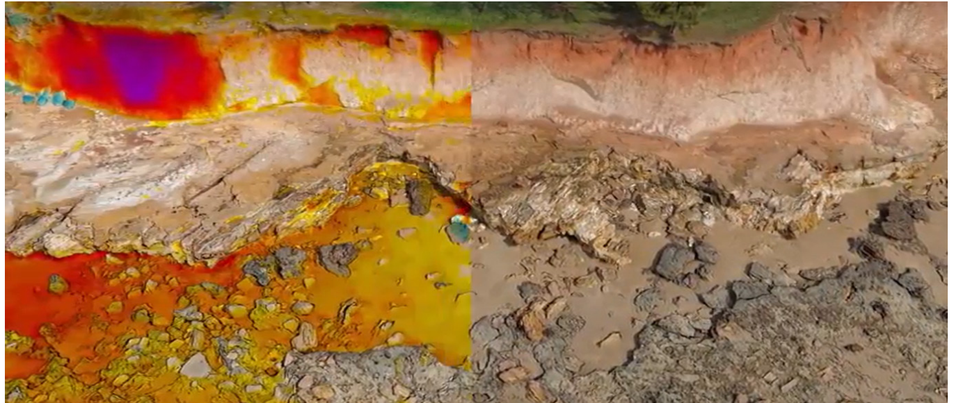
Terrain maps captured at separate intervals can be compared and changes in cliff locations can be analysed. The colours indicate where the terrain has changed as a result of erosion or other coastal processes.
