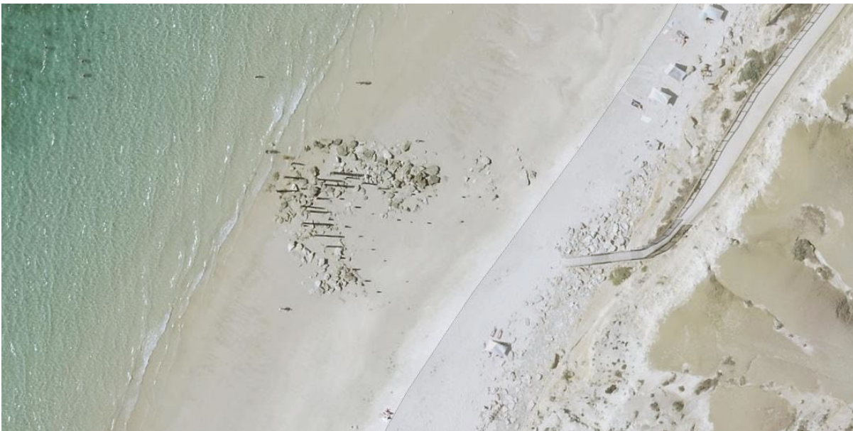
Enhancement of SAPPa satellite mapping of Port Willunga Jetty pylons, showing individual surviving pylons, associated stone foundations etc. (Planning SA SAPPa)
